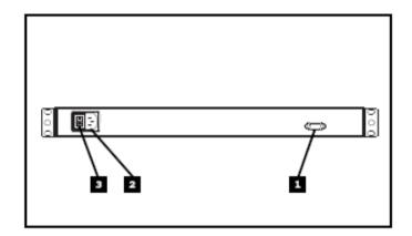
1. Console Port Section: The KVM cable kits for PS/2 or USB to connect the console to your server or KVM switch plugs in here. A console cable has been provided to connect to these ports.
